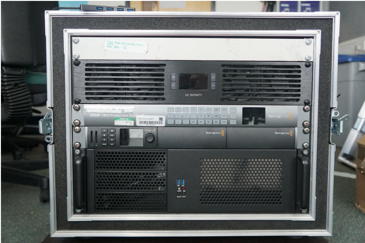
Figure 1 – The control side. Here sits the PC, ATEM and other Blackmagic components and the cooling system. A 1U gap remains at the top for future expansion.
